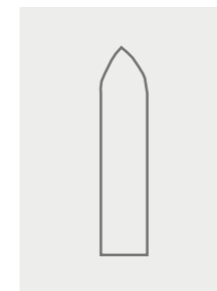
Lancet arched windows
