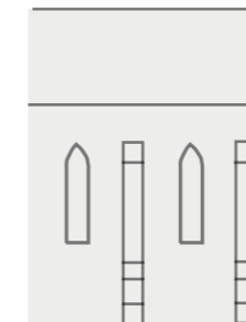
The bays are articulated with stepped buttresses.
